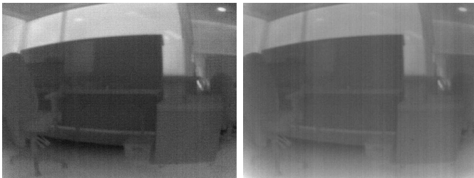
Fig. 1: Effect of the accumulation of 5 minutes of non-uniformity noise (image on the right) on the quality of thermal-infrared video. Note that non-uniformity noise is always present in thermal-infrared images. However, the right image contains much more of this noise, as it was captured much longer after the most recent NUC had been performed. The left image, in contrast, was captured only a few seconds after the NUC.
